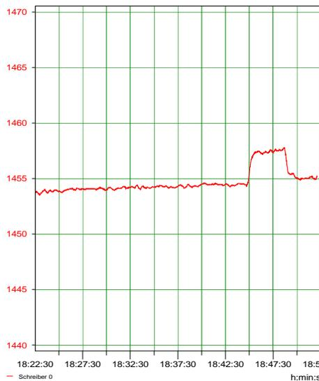
Figure 3 shows the significant increase in the speed of sound by shear stress.
