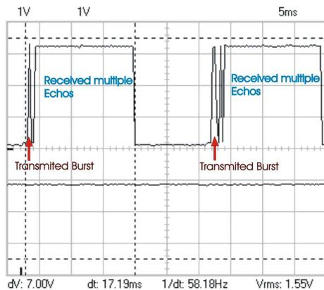
The penetration depth of process water (soapy water between the single muds) is in image (2). The distance of the transmission burst is 28 ms. The amplification of the received pulses of ultrasound was chosen so that multiple echoes not per the new transmitter into range. The process water, a penetration depth is achieved by 17,19 ms, corresponds to about 25 m or 640 inch.
