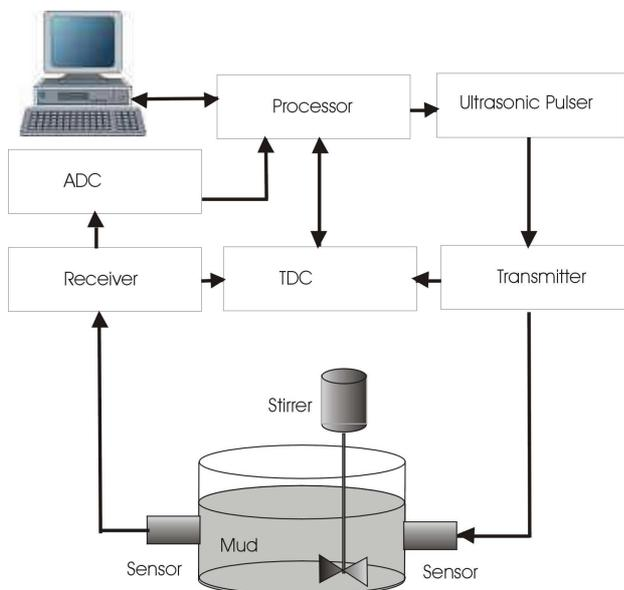
Figure (1) shows the experimental setup with a PC-controlled processor that monitors the variable burst pulse generation. Is the transit time between the transmitter and receiver with a standard deviation (time measurement) of approximately 50 ns with a TDC is determined.
